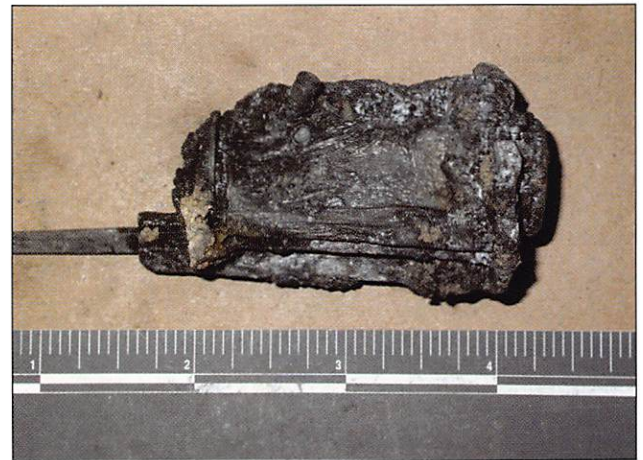
Ignition lock recovered intact from debris
