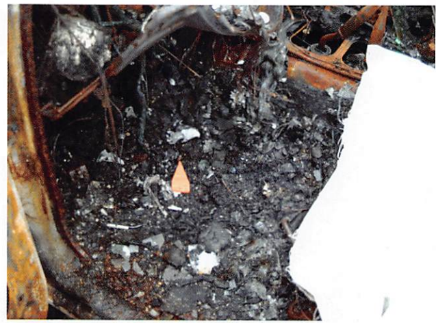
Once the large pieces of debris are cleared the smaller parts can be readily located removing thin layers one at a time
