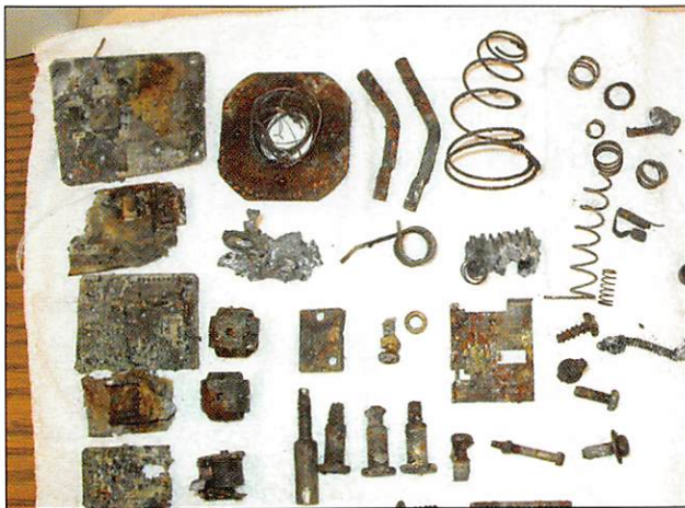
Typical debris, other than ignition lock parts recovered from a burnt vehicle. Debris generally found includes, springs, screws, relays, electrical components and a whole host of other items
